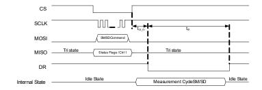
Figure 5: Timing diagram of a measurement cycle
