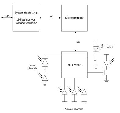
Figure 1: Rain Light Sensor system component overview
