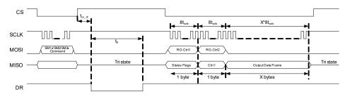
Figure 6: Timing diagram for Read-Out
