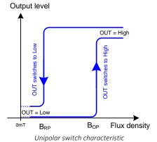
The US5683 device is inverted output, north pole active: Applying a north magnetic pole greater than  $B_{OP}$  facing the branded side of the package switches the output high.
