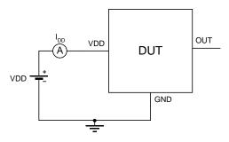
Note 1 - The supply current  $I_{\rm DD}$  represents the static supply current. OUT is left open during measurement.
