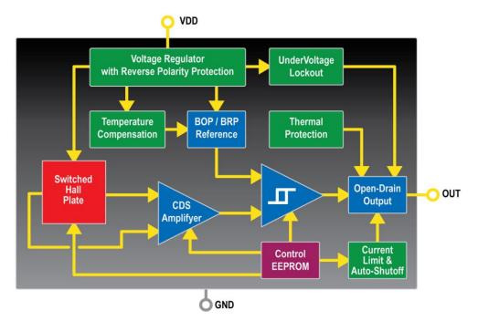
range of  $\pm 0.4$ mT to  $\pm 80$ mT and a magnetic switch range of  $\pm 1.5$ mT to  $\pm 66$ mT and a programmable hysteresis range between 1mT and 36mT. The negative thermal coefficient can be adjusted in the
